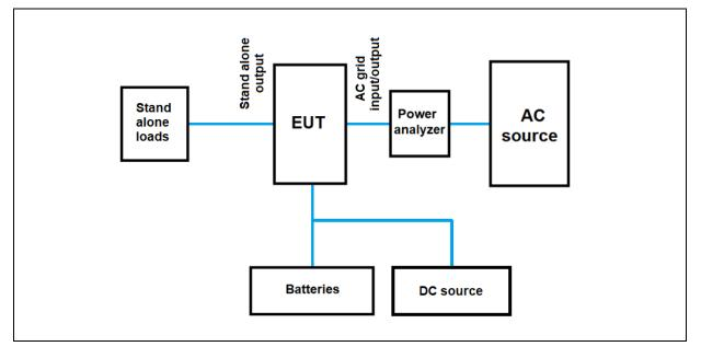
Different equipment has been used to take measures as it shows in section 2.3 of this Test Report. Current and voltage clamps have been connected to the inverter input / output for all the tests.
